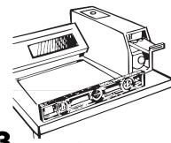
■Tilt washer forward raising back legs 1 inch off of floor. To adjust rear self-leveling legs, gently lower washer to floor. Check levelness of the washer by placing a carpenter's level on top of the washer, first side to side; then front to back.
